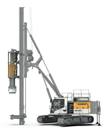
By supporting the leader on the ground and extending the rear support cylinders, the carrier machine is elevated. The undercarriage can thus be swivelled on the spot, which makes it easier to move the piling rig in restricted spaces.
